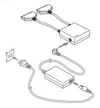
Figure 2. Connecting the AC Adapter
